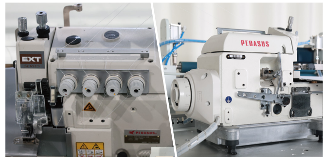
上/下机头：飞马包缝机 Upper/Lower Machine Head: Pegasus Overlock Sewing Machine
