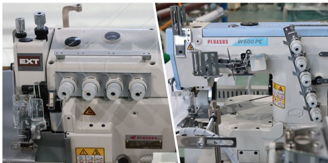
上机头：飞马绷缝机/下机头：飞马包缝机 Upper head: Pegasus Interlock Lower head: Pegasus Overlock
