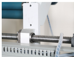
丝杠驱动 Lead Screw Drive
